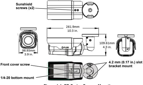
Figure 1-1: FB-Series Camera Mounting
