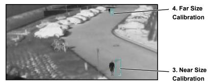
Figure 3-2: Manual Calibration
