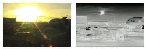
Figure 2-3: Images facing sun from standard camera (left) and thermal camera (right)
